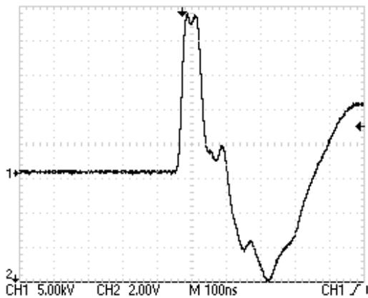
Figure Xe. Laser Drive 7500 P.S. Trigger Pulse (no load)
