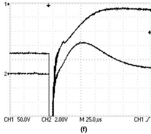
Figure Z. Boost Voltages & Currents: (a) Laser Drive 040-75150, (b) EMSC P.S. operating @ 125 Watts, (c) EMSC P.S. operating @ 300 Watts, (d) Rotec ECG300 Xe P.S., (e) Rotec ECG300 DC HE P.S., (f) Laser Drive 7500 P.S.
