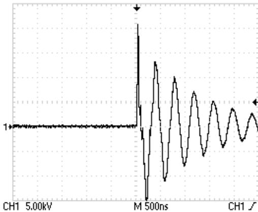
Figure Xc. Rotec ECG300 DC HE P.S. Trigger Pulse (no load)
