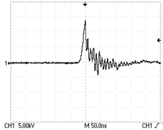
Figure Xb. Rotec ECG300 Xe P.S. Trigger Pulse (lamp connected)
