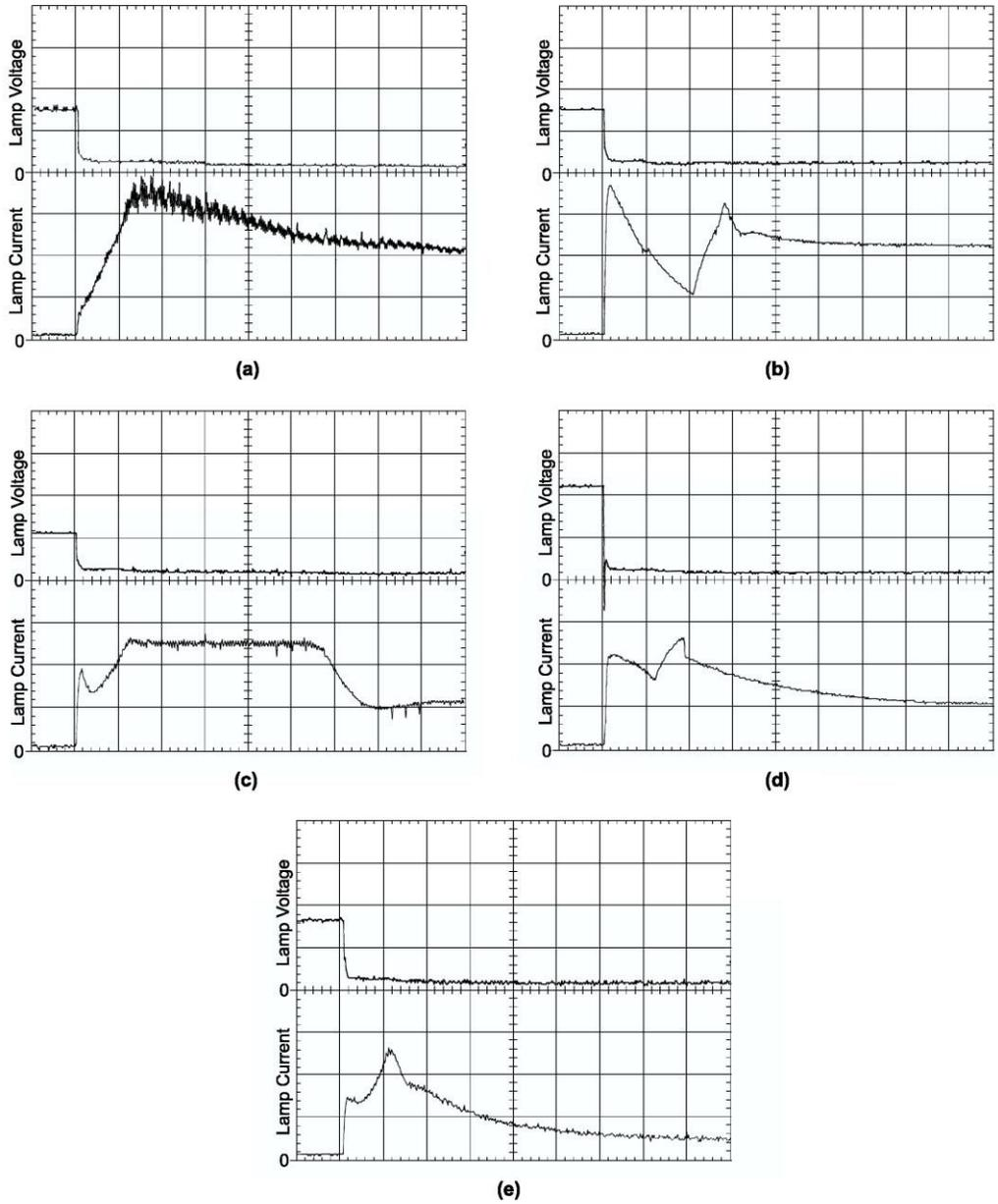
Figure AA. Additional Boost Voltages & Currents of older power supplies, Time Base is 500 msec. per division, Boost Voltage set at 100 volts per division. (a) PS1 75 SW-1 Power Supply (10 Amps / div.), (b) PSC300 (10 Amps / div.), (c) PS300 SW-2 (20 Amps / div.), (d) PS 300-1 linear supply (20 Amps / div.), (e) PS500 -10 (50 Amps / div.)
