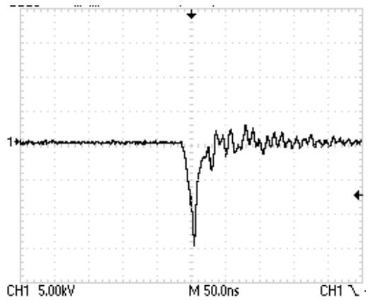
Figure Xd. Rotec ECG300 DC HE P.S. Trigger Pulse (lamp connected)
