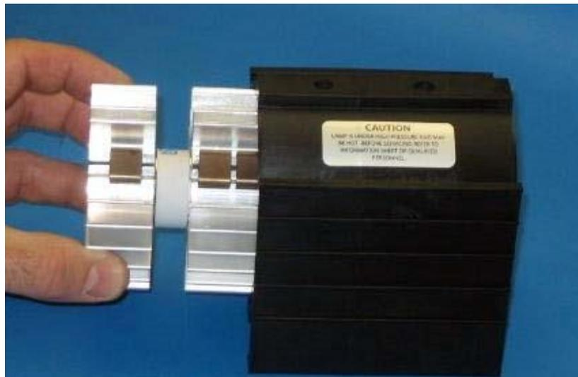
Step 3: Slide lamp and heatsinks out of module.
