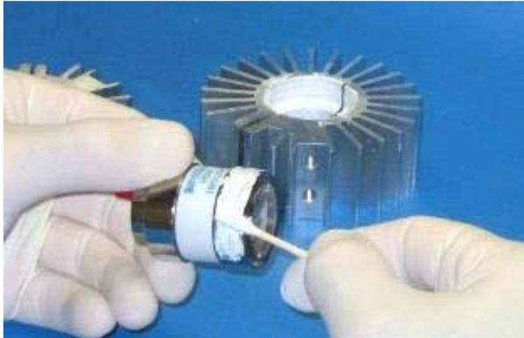
Step 10: Apply a thin layer of thermal compound to the outer band of the cathode end of the lamp. Apply compound to outer diameter of cooling ring (if not already seated in heatsink). Take care not to apply compound to the window or ceramic surfaces. Any compound should be removed with the use of alcohol and wipes.
