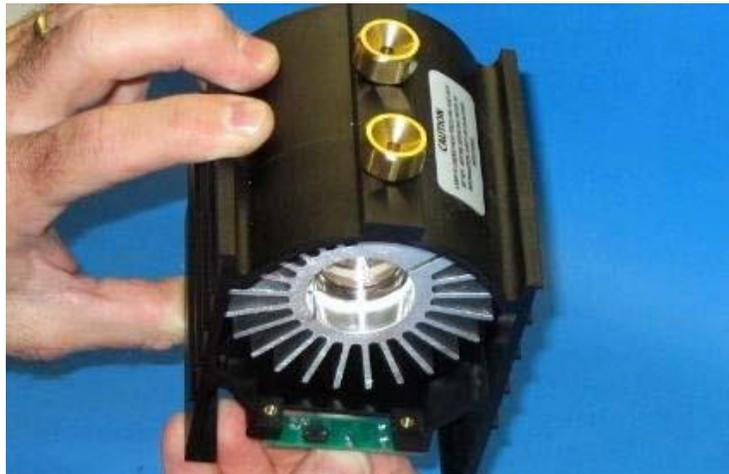
Step 18: If using optional photodiode timer assembly, mount as shown with photodiode facing up and printed circuit board mounted from the bottom. Scaled hour meter is on opposite side of board.
