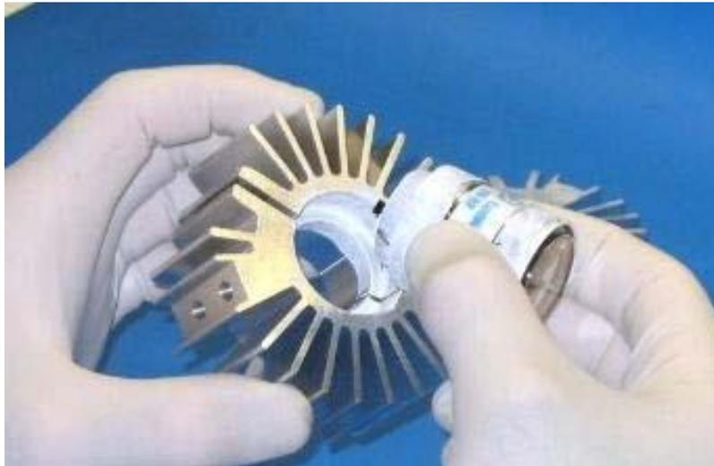
Step 8: Remove old lamp from heatsink assemblies and set aside.
