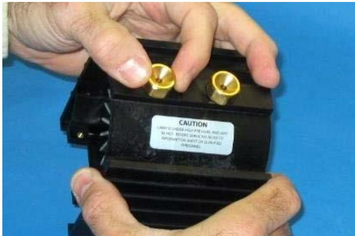
Step 17: Insert brass connectors through housing and into heatsinks. Note that the 10-32 threaded connector goes into the anode/rear heatsink and the 8-32 threaded connector is for the front/cathode heatsink. Connectors may be secured tightly by hand. If tightened with a wrench, use a torque wrench and do not exceed 16 in-lbs.
