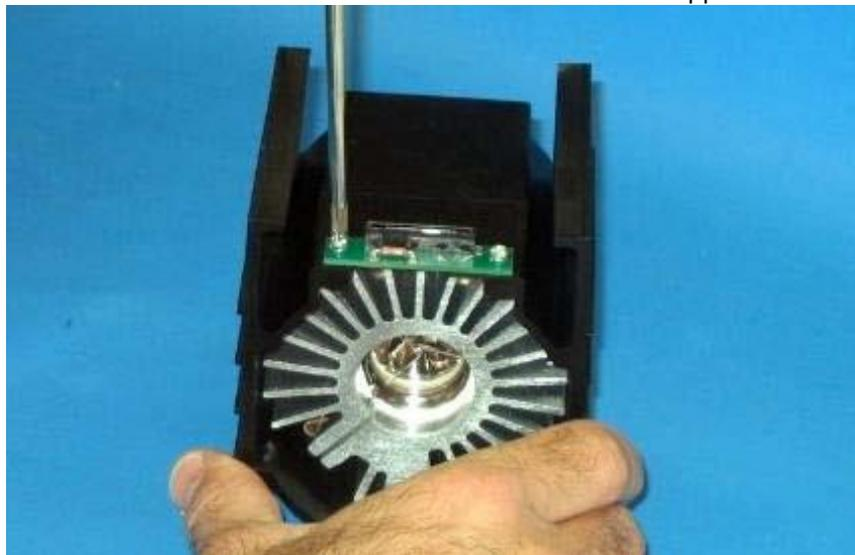
Step 19: Align mounting holes in printed circuit board with threaded inserts in housing and secure with two 4-40 x 1/4" screws.
