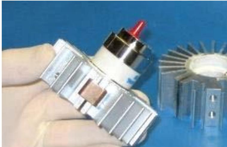
Step 12: Orientation of the lamp may occur at this time, if desired. Place one spring clip on cathode heatsink until fully seated.
