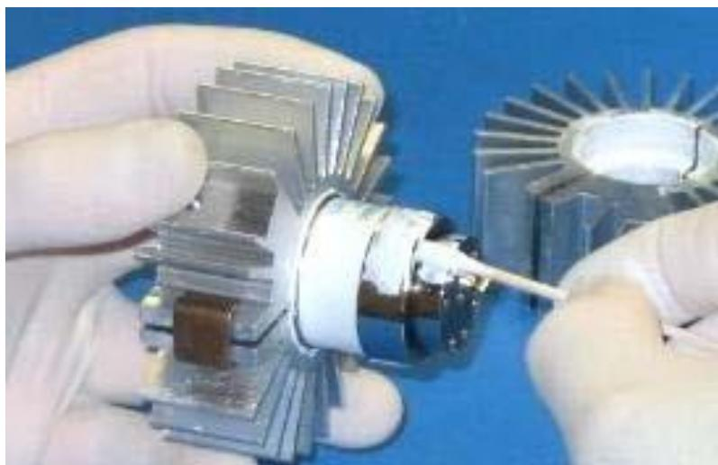
Step 14: Apply compound to the outer band and diameter of the anode base. Take care not to damage the pinch off seal.
