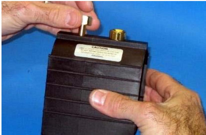
Step 2: Remove both brass electrical connectors and set aside.
