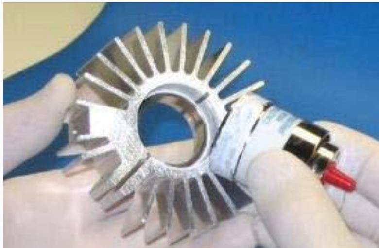
Step 11: Insert the cathode end of the lamp into the cathode heatsink and rotate. Assure that the lamp is fully seated in the cooling ring and heatsink. Metal band of lamp should not be visible when properly seated.
