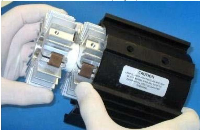
Step 16: Insert lamp with heatsinks into the housing assuring that the window/cathode end is facing the housing end with cut out that holds optional timer assembly.
